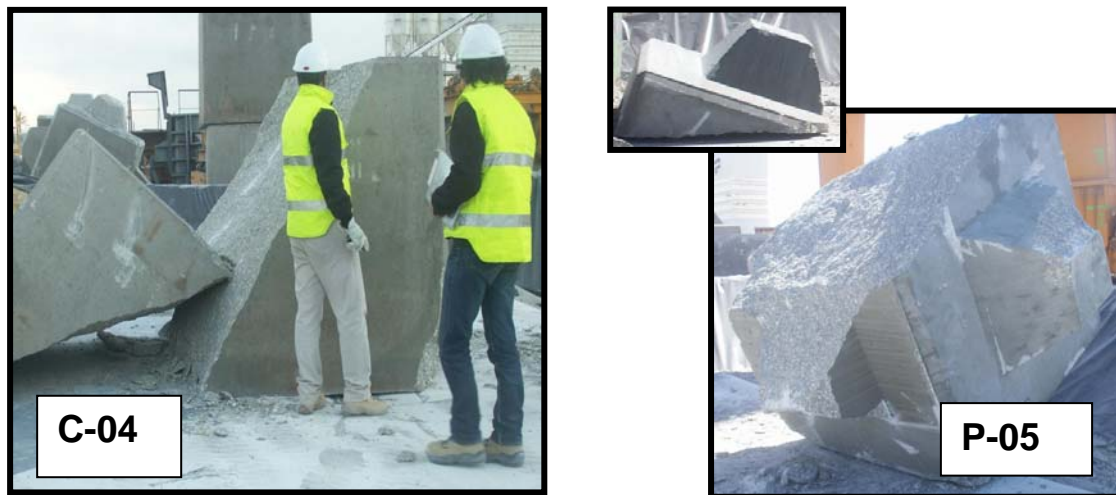
Figure 9. Fracture planes of broken cube and Cubipod prototypes.
