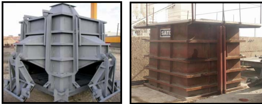
Figure 1. Pictures of prototype casting systems: (a) Cubipod and (b) cube.
