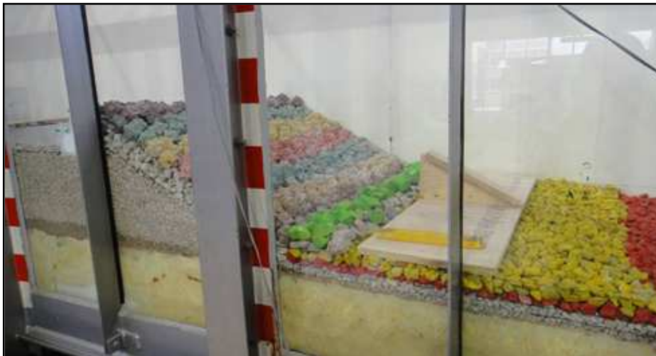
Figure 2. Single-layer Cubipod armor in 1/40 scaled model at UPM wave flume.
