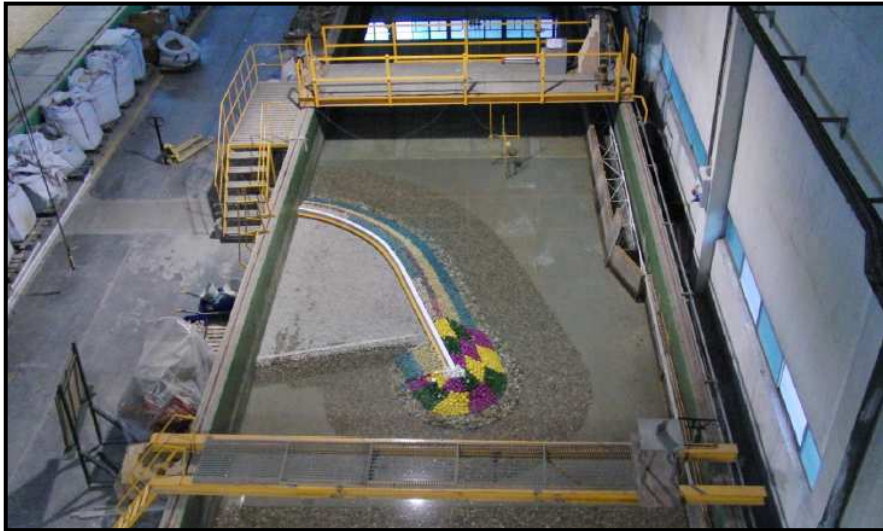
Figure 3. Double-layer Cubipod armor in 1/36 scaled model at CEDEX wave basin.
