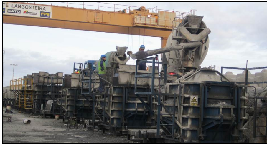
Figure 7. Production line of 25-tonne Cubipod units.
