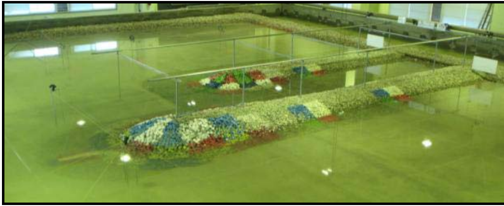
Figure 3. 3D wave basin and 1/45 -scale model with double-layer 5-tonne quarrystone and double-layer 20-tonne and 35-tonne cube armors.
