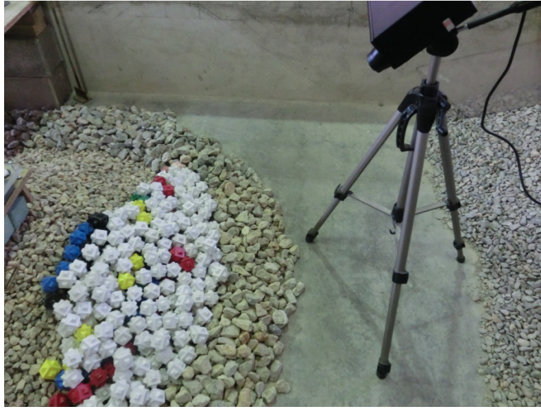
Figure 5. Laser scanning process for a Cubipod armor.
