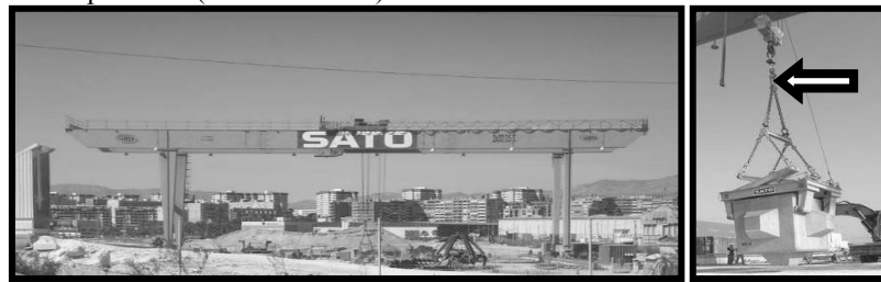
Figure 8. Port of Alicante: (a) gantry crane and (b) double tong with load cell.
