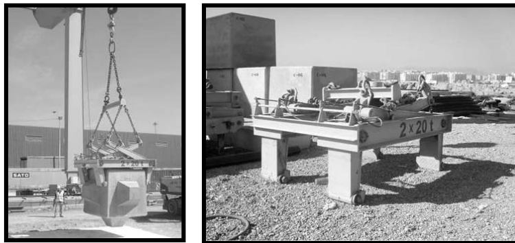
Figure 6. Double tongs adapted to handle prototype Cubipods.
