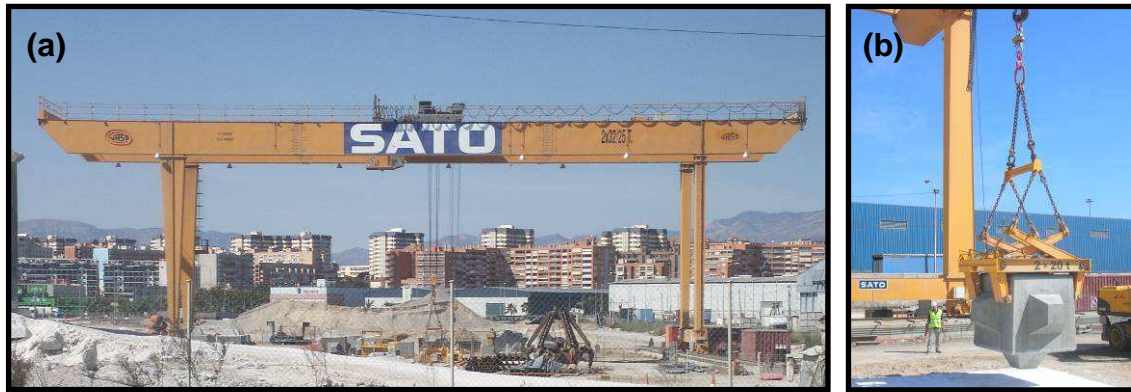
Figure 5. (a) 63/25-tonne gantry crane and (b) double tongs used to handle Cubipods.
