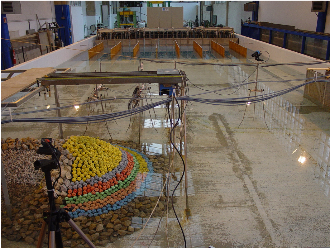
Figure 2: Photograph of the wave basin and the roundhead Cubipod model during testing.
