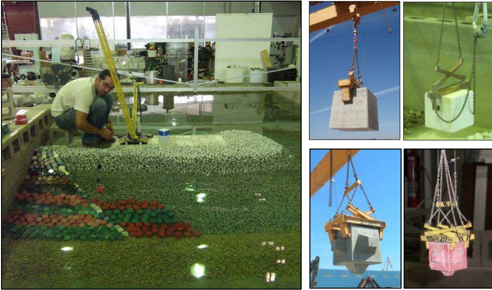
Figure 6. 3D placement test, small-scale crawler crane and pressure clamps.
