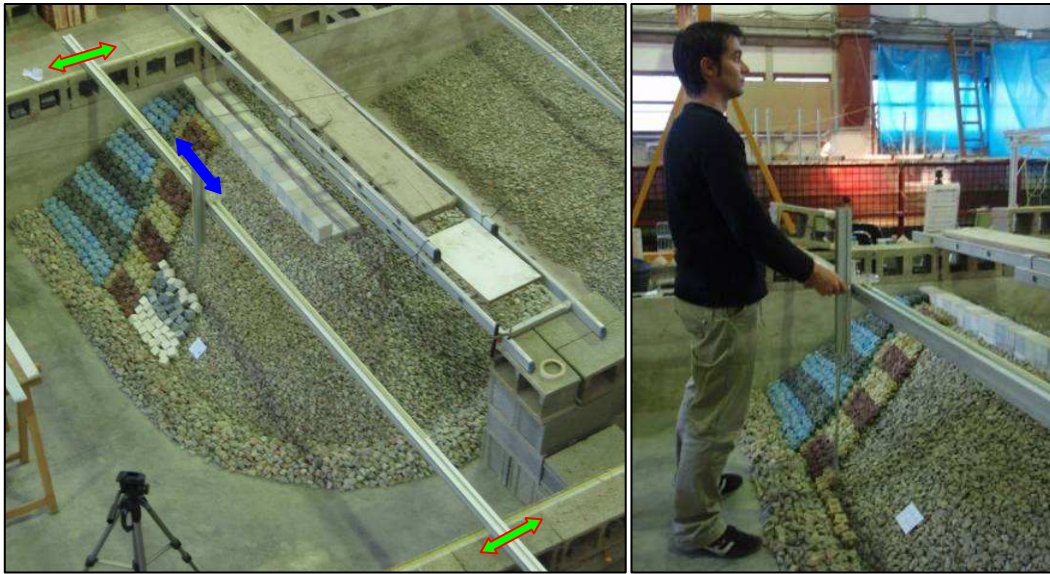
Figure 9. Views of Cartesian Blind Placement System (left) and clamp operator (right).
