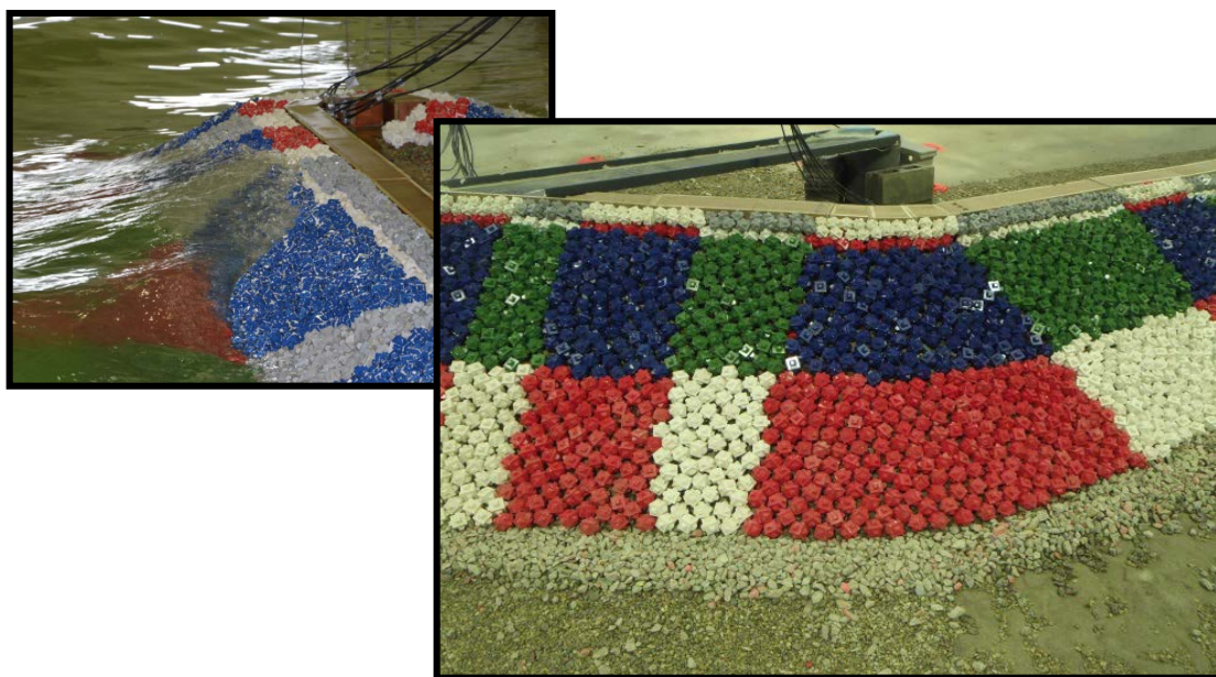
Figure 3. Roundhead testing, and curved trunk after wave attack H_s(m)=9.0 .
